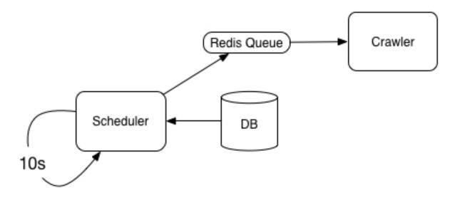
The scheduler allows for scheduling certain type of jobs such as crawling jobs for the feeds. This is really just a simple piece that create a set of tickets for crawling (FeedCrawlingRun) and queues them for processing in a Redis queue. This enables an automated recurring scheduler or manual scheduling of a crawling. (Just inject the ID into the queue for processing.)
