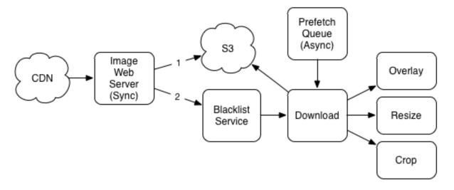
Process for Image Request: An Image request is sent to our image web service (either by the CDN or directly by a user.)
